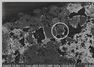
Fig. 5 SEM image of the cross-section in Fig. 4. The white circle marks a characteristic vanadinite crystal formation.
