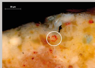
Fig. 4 Micrograph (DIC) of a cross-section representing the pale, greenish yellow paint on one of the leaves. The white circle marks a characteristic vanadinite crystal formation.
