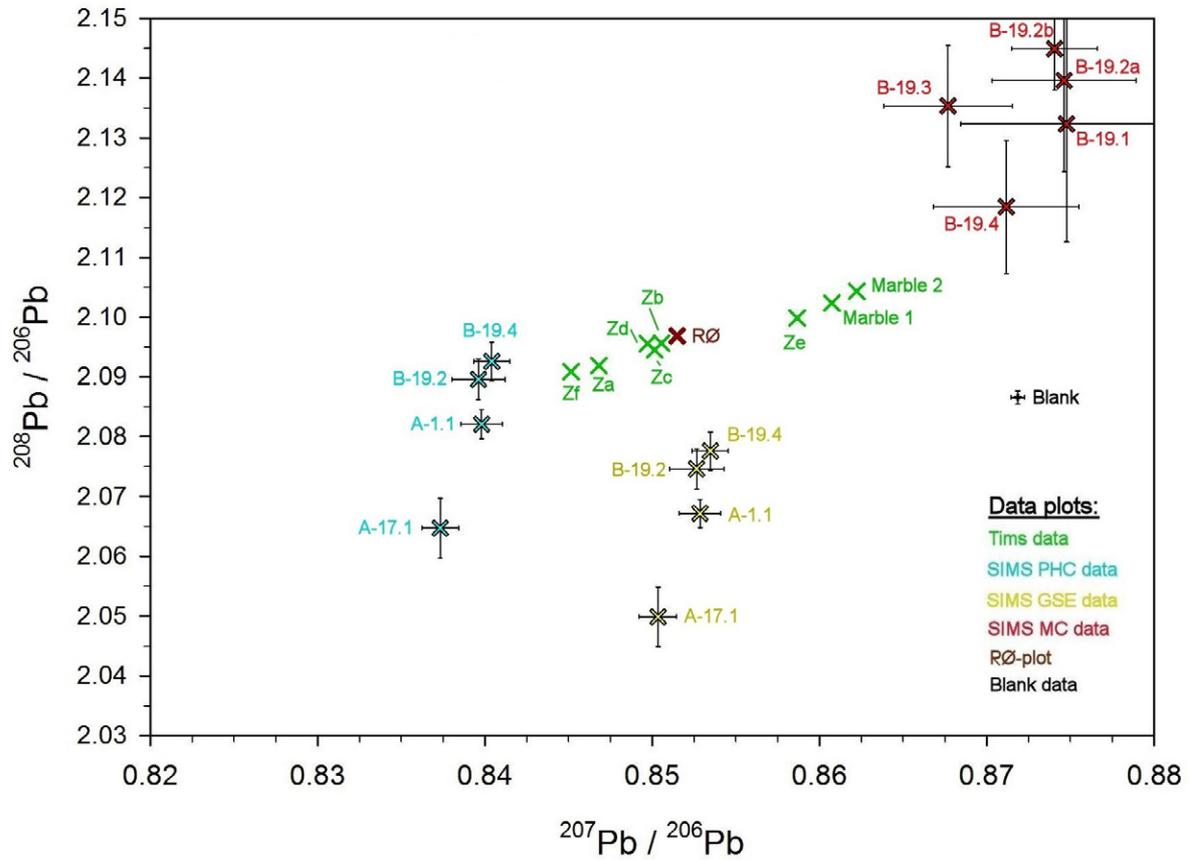
Fig. 7: Data from SIMS and TIMS analyses plotted in a  $^{208}\text{Pb}/^{206}\text{Pb}$  vs  $^{207}\text{Pb}/^{206}\text{Pb}$  diagram. SIMS data plots are presented with  $2\sigma$  error bars. Error bars for TIMS data are not shown as the standard deviation values are insignificantly small. The RØ data plot is taken from Rosing
