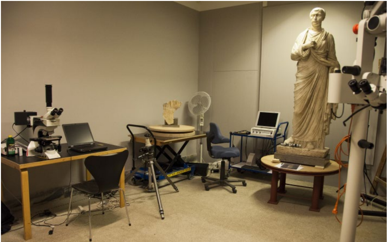
Fig. 1: The new work space is a c. 25 sqm room with access conditions and ceiling height permitting investigation of full size sculptures. On the heavy duty turntable is the portrait statue of Fundilia from Nemi, IN 708: on the smaller turntable mounted on a hydraulic lift table is the Egyptian limestone relief fragment ÆIN 1048. Between the two is the Leica DVM 5000 video microscope. On the left is the Leica 2500 optical microscope, on the right a glimpse of the Leica M65 operations microscope. The space is equipped for all types of technical, analytical photography.
