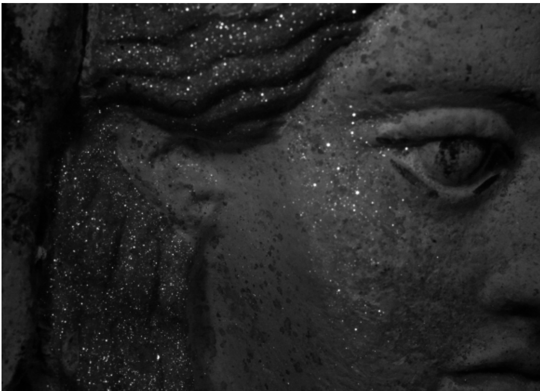
Fig. 22: vIL-image of the face of HIN 453 showing the distribution of Egyptian blue as shining white particles both on the skin and in the hair.
