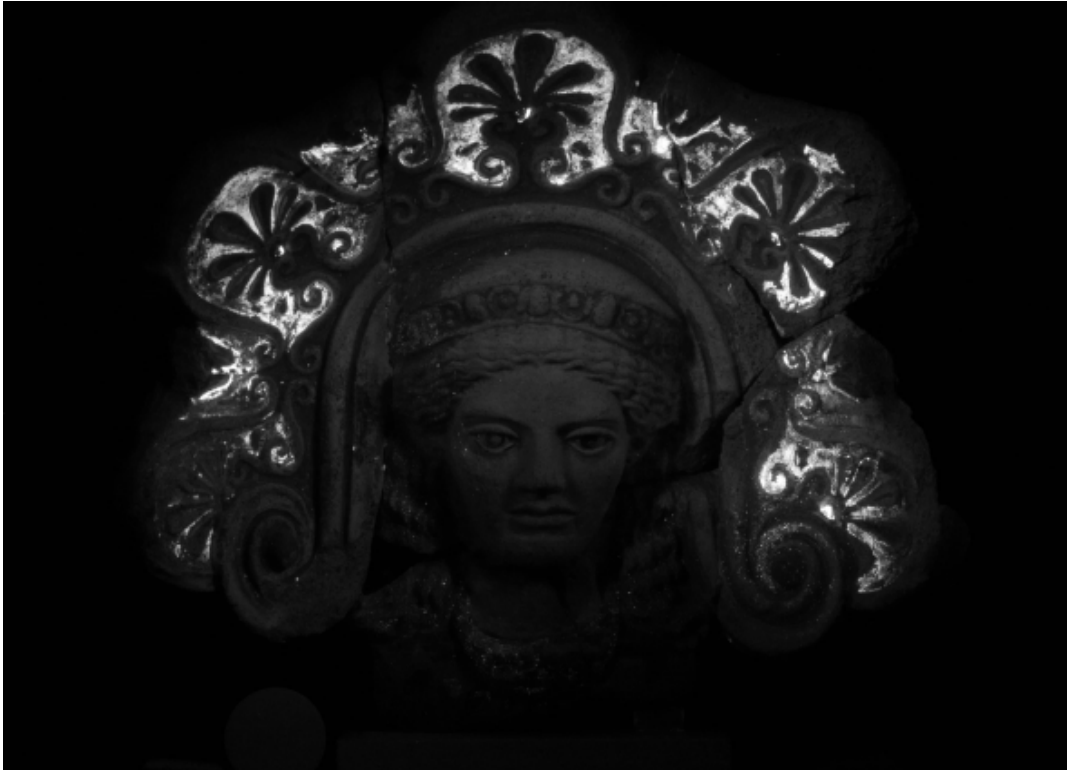
Fig. 10: vIL-image of HIN 452 showing the distribution of Egyptian blue as shin- ing white areas.
