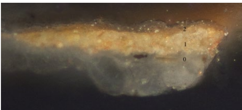
Fig. 16: Micrograph of polished cross-section of sample showing the stratigraphy of the skin colour on IN 2815. On top of the marble (0) a yellowish layer with a few red grains was observed (1). On top of this is a thin, reddish layer (2). The second layer was partly covered by incrustation, ×200.
