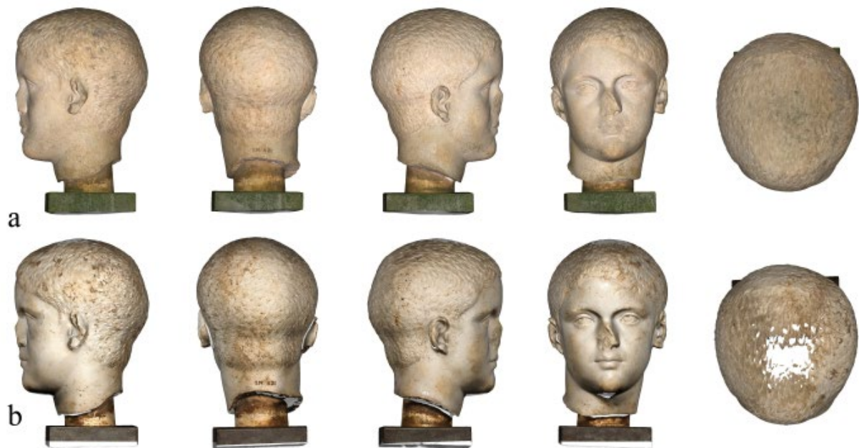
Fig. 4: Color projection strategies. a. vertex attribute transfer in MeshLab, b. texture mapping in MeshLab.
