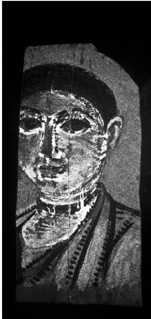
Fig. 8: As fig. 7. Visible-induced luminescence (VIL) image showing the spatial distribution of Egyptian blue, appearing bright white.
