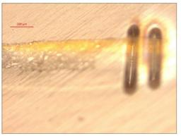
We used a Jena/Bruker M90 Aurora ICP-MS with a CETAC LS-213 Laser Ablation input operated at 10 Hz and 85 % laser power. The data are not yet quantified.
